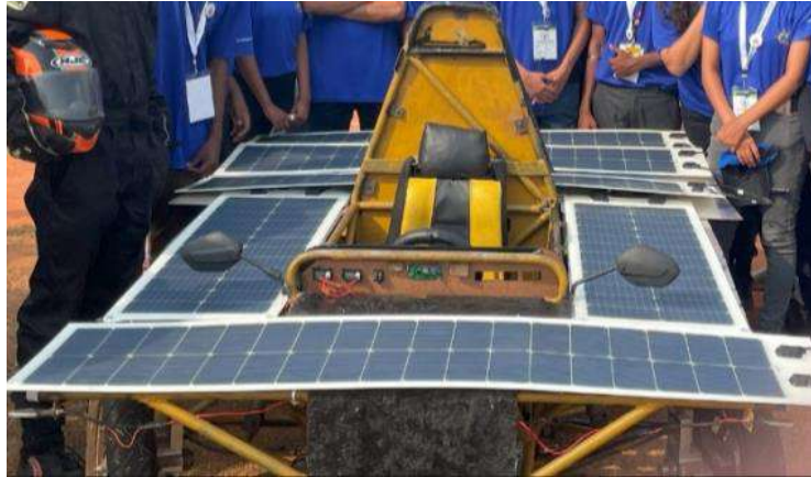
Figure 4: Solar panels integrated with the solar vehicle
