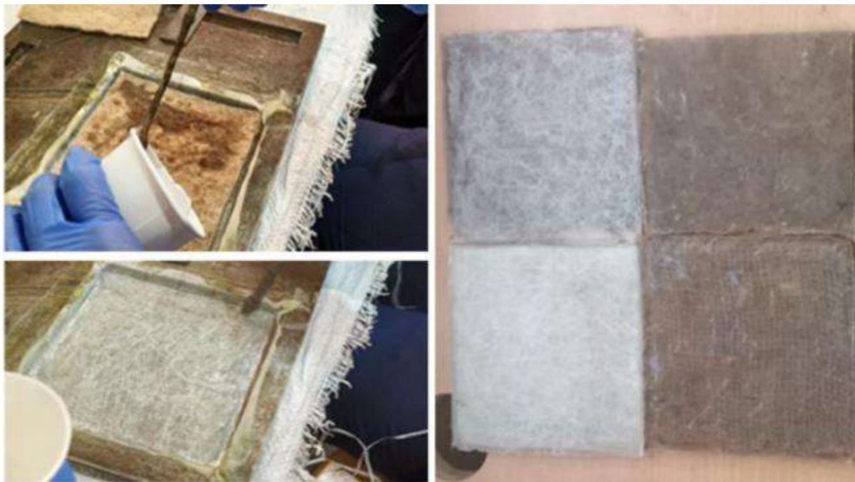
Figure 3: Hand layer process used in the preparation of different eco-friendly fiber samples
