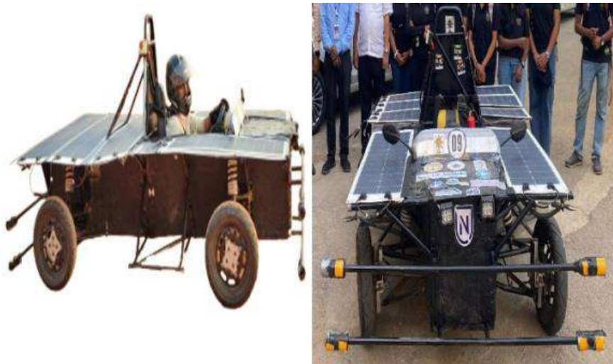
Figure 8: Glimpse of developed Electric vehicle powered by Solar energy
